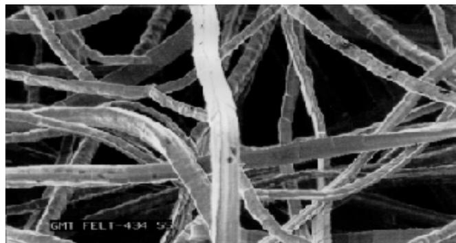
100x Micrograph of 40µm Stainless Steel Fibers
